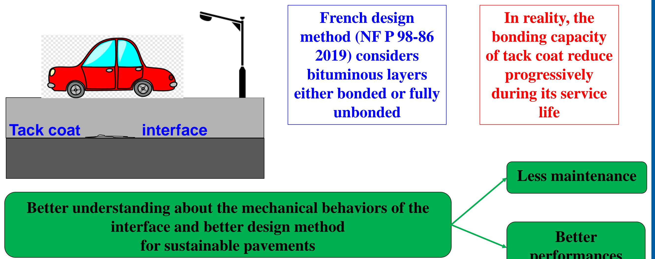
OBJECTIVE: characterize interface between bituminous layers under shear loading in Linear Viscoelastic (LVE) and fatigue domains by using 2T3C (Torsion/Traction/...) apparatus developed at ENTPE (Attia, 2020)
